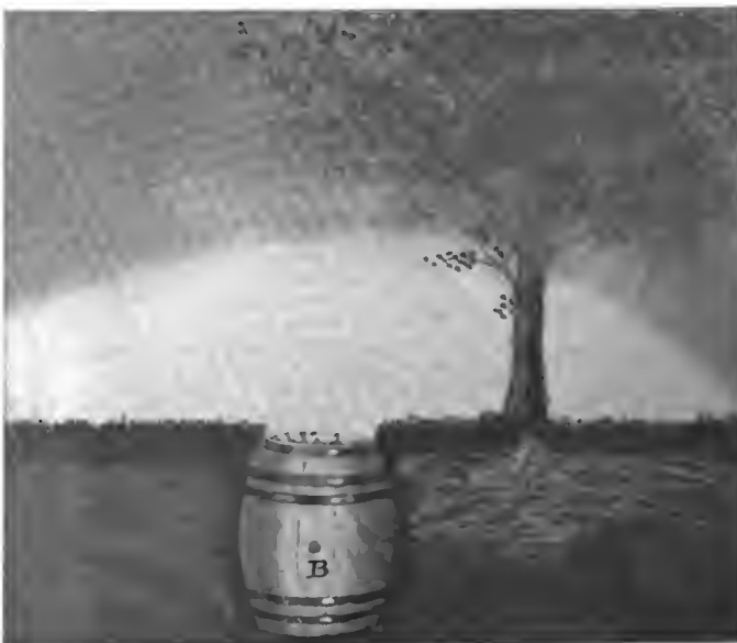
Fig. 7—Barrel of gasoline sunk in the ground, leaking gasoline to the surrounding, as the liquid evaporates and mixes with the air surrounding it lifts the fog by displacement
